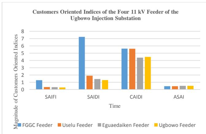
Figure 6: Customers Oriented Indices of the Four 11 kV Feeders of Ugbowo 2x15 MVA, 33/11 kV Distribution network
