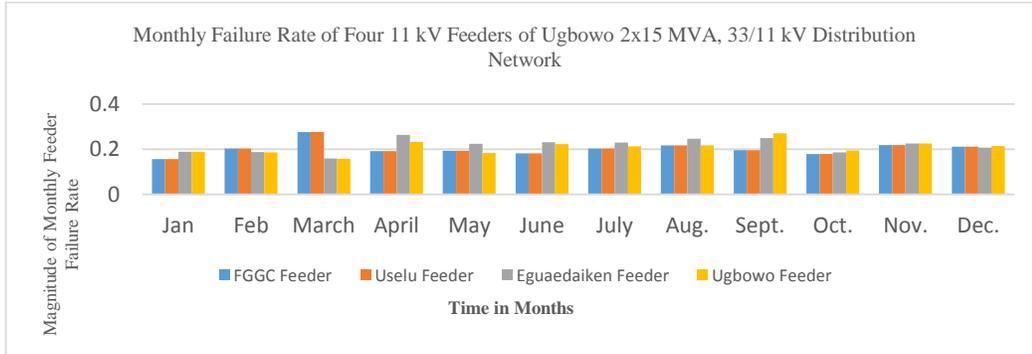
Figure 2: Monthly Failure Rate of 11 kV Feeders of Ugbowo 2x15 MVA, 33/11 kV Distribution Network
