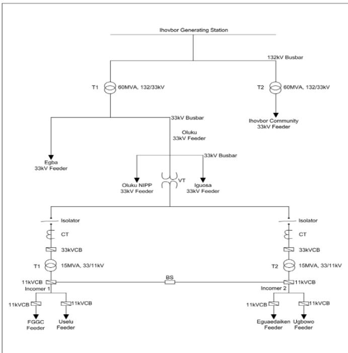
Figure 1: Single Line Diagram (SLD) of the Ugbowo 2x15 MVA, 33/11 kV Distribution Network feeders and the 132/33 kV Supply from Ihovbor Generating Station.
