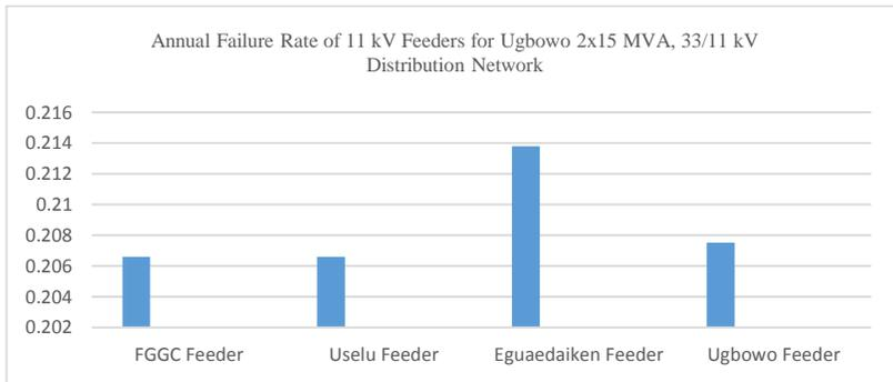
Figure 2: Annual Failure Rate of 11 kV Feeders of Ugbowo 2x15 MVA, 33/11 kV Distribution Network
