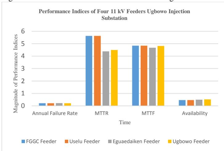
Figure 5: Performance Indices of Four 11 kV Feeders of Ugbowo 2x15 MVA, 33/11 kV Distribution Network.
