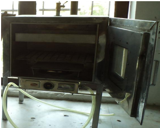
Fig 6. Fabricated Electric/Coal/Gas Oven
