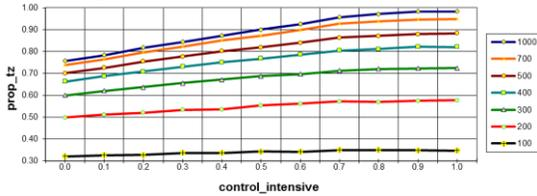
Fig.6: Dependence of probability of timely delivery of messages on the intensity of controlling for different values of tz, specified time
