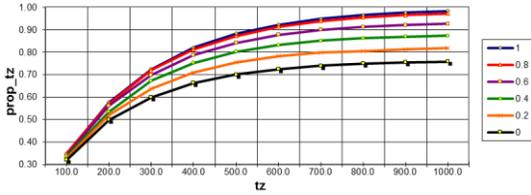
Fig. 7: Dependence of probability of timely delivery of messages on specified transmission time for different values of intensity of controlling, control\_intensive
