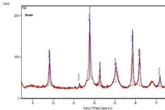
Figure 2: XRD of MgO Nanoparticles
