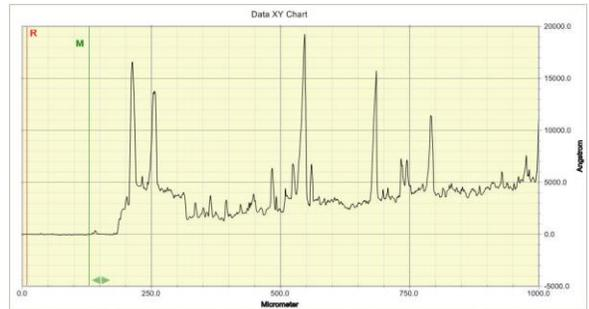
Figure 7: Surface Profiler showing the film thickness for RGO\_HI\_RC
