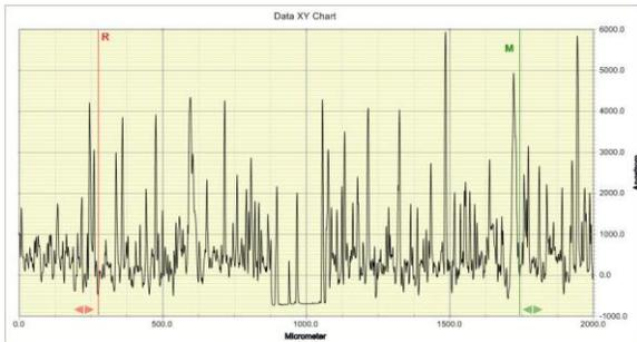
Figure 4: Surface Profiler showing the film thickness for GO
