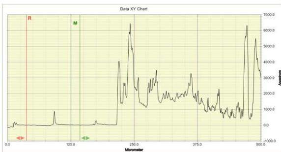
Figure 6: Surface Profiler showing the film thickness for RGO\_HI
