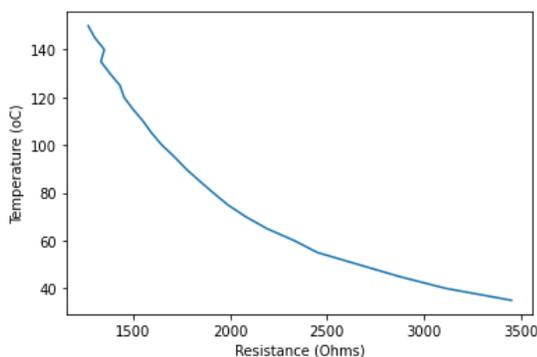
Figure 9: T-R characteristics of the Heat Sensor
