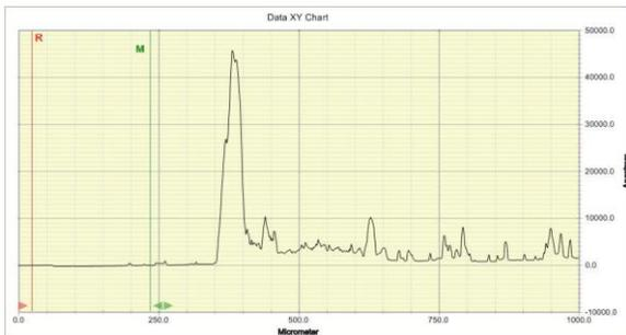
Figure 8: Surface Profiler showing the film thickness for RGO\_HYD
