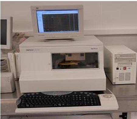
Figure 2: An image of a Profilometer Machine
