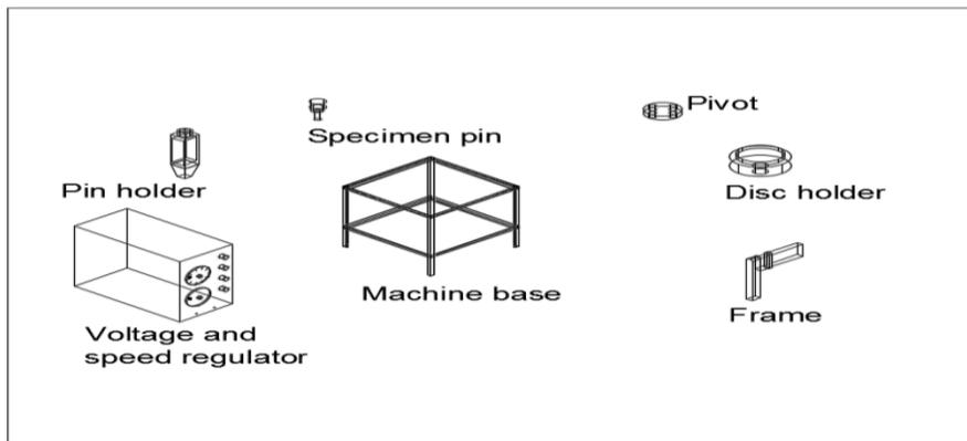
**Figure 2: Components of the Pin on disc machine**
