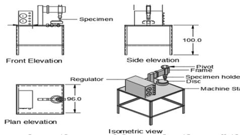
**Figure 1: Third angle orthographic projection of the Pin on disc machine**
