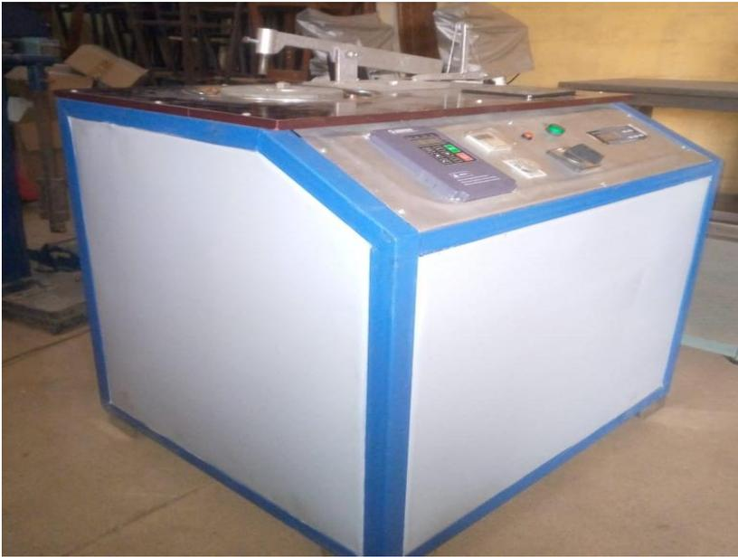
**Figure 3: The Constructed Pin on disc wear test machine**
