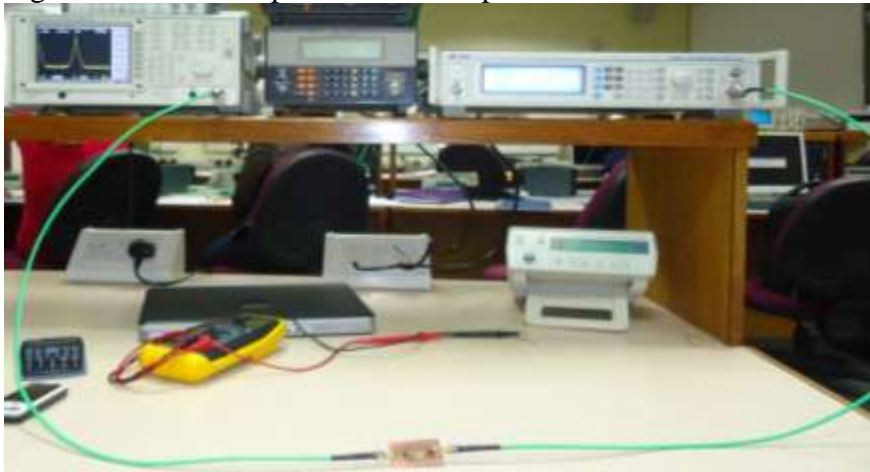
Figure 3.0: Testing Setup of the 3.4 \text{ MHz} Microstrip Bandpass Filter Design Implementation
