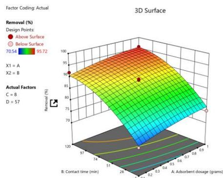
Figure 10: Contact time and adsorbent dosage relationship 3D
