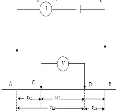
Figure 2: Geometry for Schlumberger configuration
