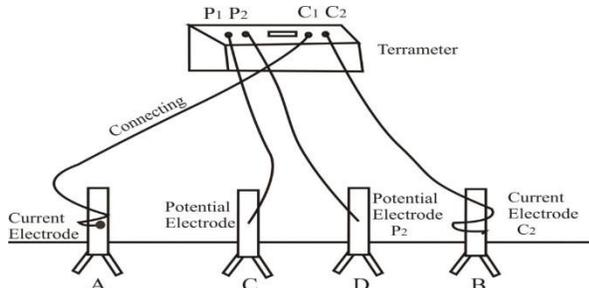
Figure 3: Schematic diagram of the Schlumberger array.
