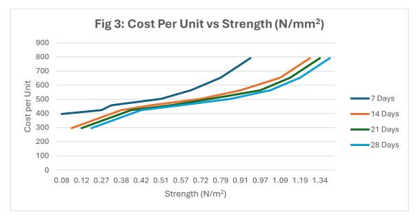
Cost per unit correlated in same direction as ultimate failure strength in compression (Figure 3). It shows that as cost of batching increased, strength increased also. A maximum strength of 1.404N/mm<sup>2</sup> was got at 28 days curing age while the minimum for same age was 0.122N/mm<sup>2</sup> corresponding to 791.65 naira and 396.57 naira respectively.
