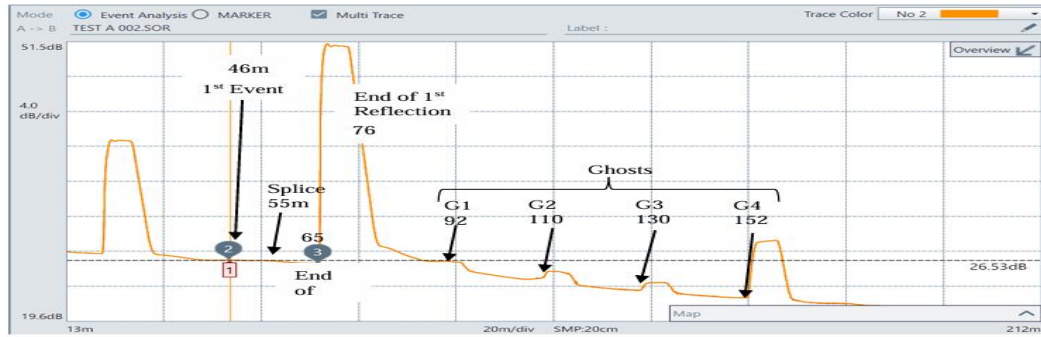
Figure 4.2: Full OTDR trace of SMS fiber with 50 ns pulse width at 1550 nm at low temperatures (-0.3°C to 7.9°C).
