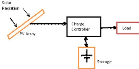
Figure 1: Block diagram of typical stand-alone (off-grid) PV system.
