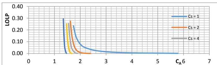
Fig. 5 Variation of LOLP with array capacity  $C_A$  at various storage capacities  $C_S$  for Port Harcourt.
