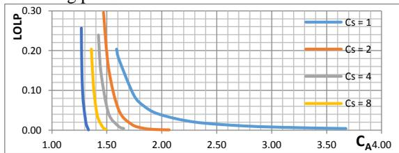
Fig. 3 Variation of LOLP with array capacity  $C_A$  at various storage capacities  $C_S$  for Lagos.
