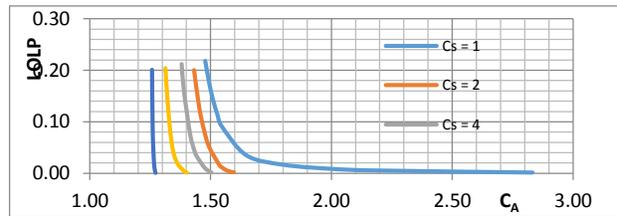
Fig. 4 Variation of LOLP with array capacity  $C_A$  at various storage capacities  $C_S$  for Abuja.
