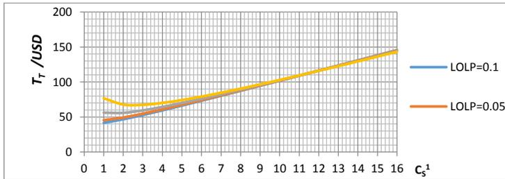
Fig. 9 Illustration of equation (19) showing variation of total system cost with storage capacity.
