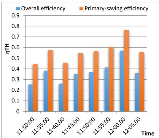
Fig. 4a - Variation of overall energy and primary-saving energy efficiencies at flow rate (a)  $\dot{v} = 10.81\text{ml/s}$
