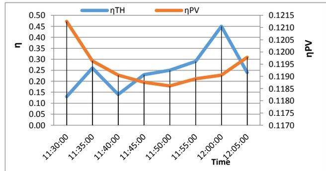
Fig. 3a - Variation of thermal and electrical efficiencies at flow rate  $\dot{v} = 10.81\text{ml/s}$
