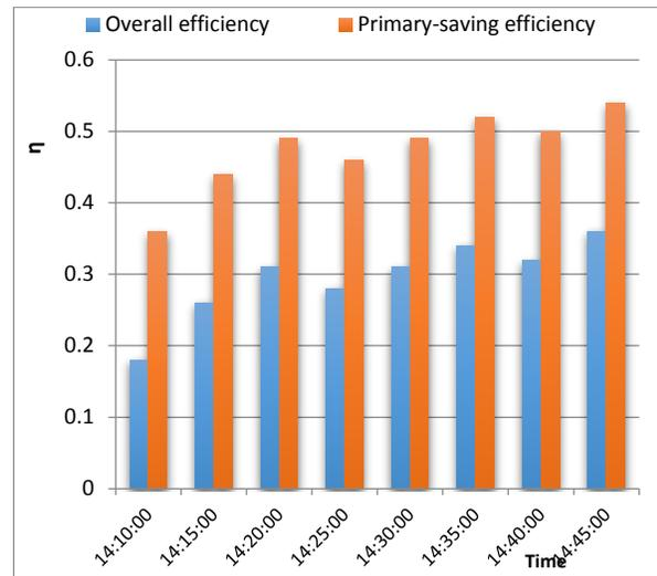
Fig. 4e - Variation of overall energy and primary-saving energy efficiencies at flow rate  $\dot{v} = 5.53 \text{ ml/s}$
