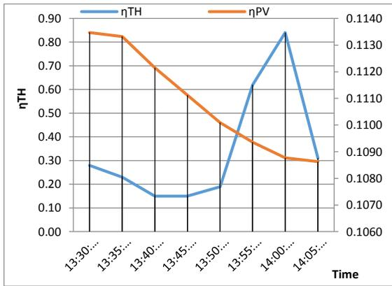
Fig. 3d - Variation of thermal and electrical efficiencies at flow rate  $\dot{v} = 20.83\text{ml/s}$
