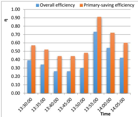
Fig. 4d - Variation of overall energy and primary-saving energy efficiencies at flow rate  $\dot{v} = 20.83 \text{ ml/s}$
