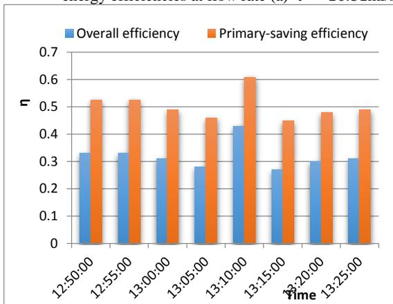
Fig. 4c - Variation of overall energy and primary-saving energy efficiencies at flow rate  $\dot{v} = 15.98\text{ml/s}$
