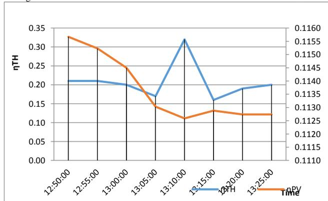
Fig. 3c - Variation of thermal and electrical efficiencies at flow rate  $\dot{v} = 15.98\text{ml/s}$
