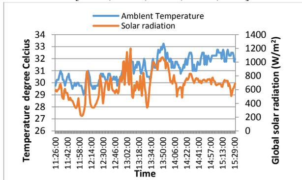
Fig. 2. Measured values of Ambient temperature, and global solar radiation.
