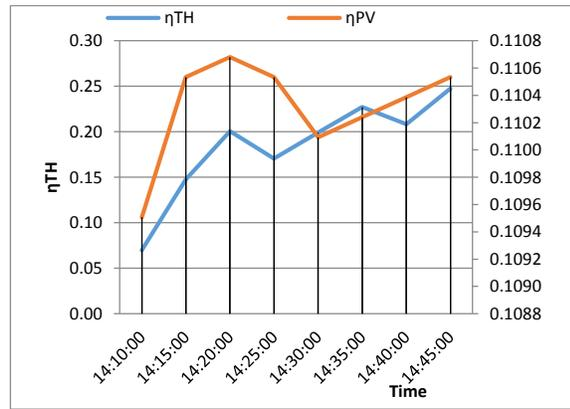
Fig. 3e - Variation of thermal and electrical efficiencies at flow rate  $\dot{v} = 5.53\text{ml/s}$
