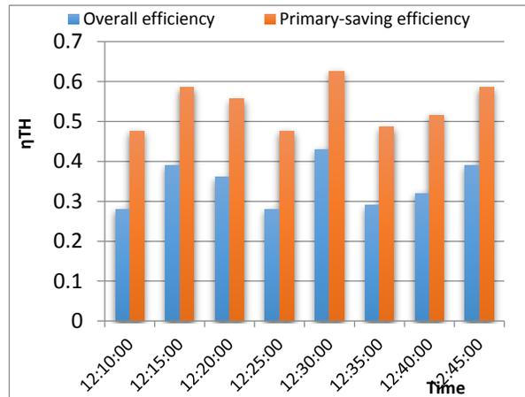
Fig. 4b - Variation of overall energy and primary-saving energy efficiencies at flow rate  $\dot{v} = 13.04\text{ml/s}$
