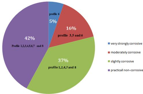
**Figure 1.10 Soil Corrosivity Rating**
