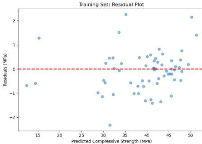
Figure 11: Plot showing the residuals i.e. the difference between the actual compressive strength and the predicted compressive strength for the training dataset of the RF regression model
