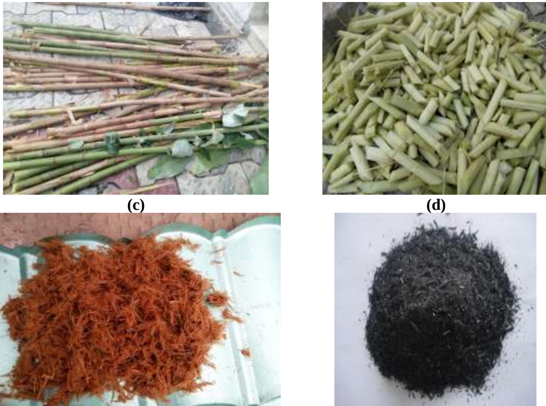
Figure 2: (a) Harvested Costus afer plant (b) Peeled and cut stems of Costus afer plant (c) Pulverized Costus afer fibre (d) Costus afer ash
