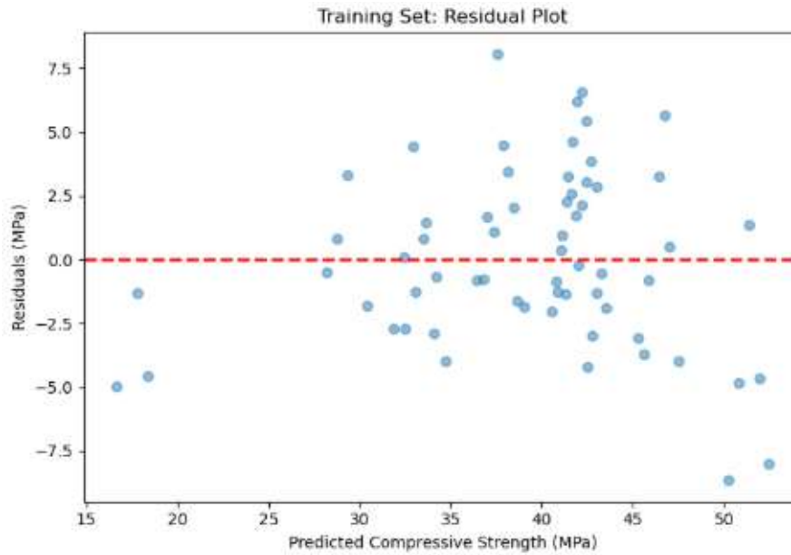
Figure 7: Plot showing the residuals i.e. the difference between the actual compressive strength and the predicted compressive strength for the training dataset of the MLR model
