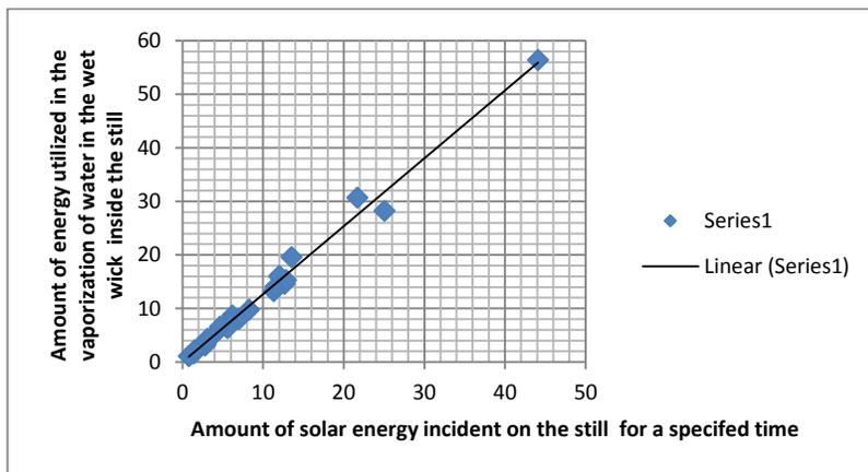
Figure 3 above: shows the relation amount of energy utilized in the vaporization of water and amount of solar energy incident on the still
