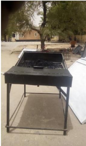
FIG. 1: A picture of wick tilted solar still
