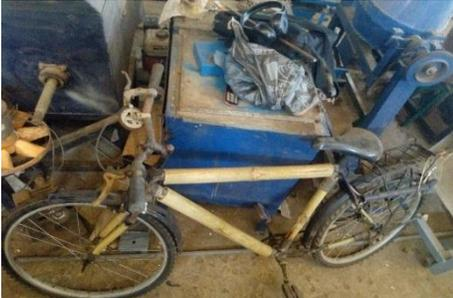
Figure 3: Bamboo made Bicycle Structure
