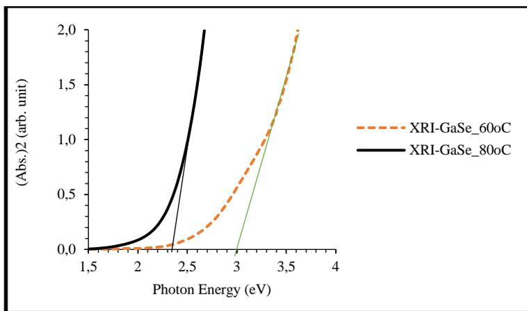
**Figure 4:** Energy bandgap estimation of X-ray irradiated GaSe thin films grown at 60 and 80°C.
