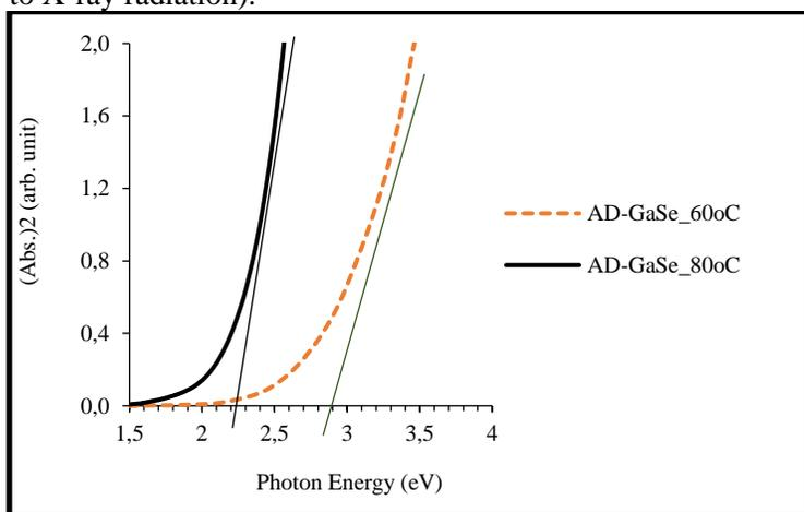
**Figure 3:** Energy bandgap estimation of as-deposited GaSe thin films grown at 60 and 80°C.
