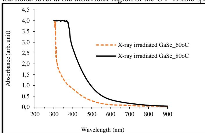
**Figure 2:** Optical absorbance graphs for X-ray irradiated GaSe thin films. (Note that the noise level at the ultraviolet region of the UV-visible spectrum has been eliminated as a result of the surface treatment of GaSe films via exposure to X-ray radiation).
