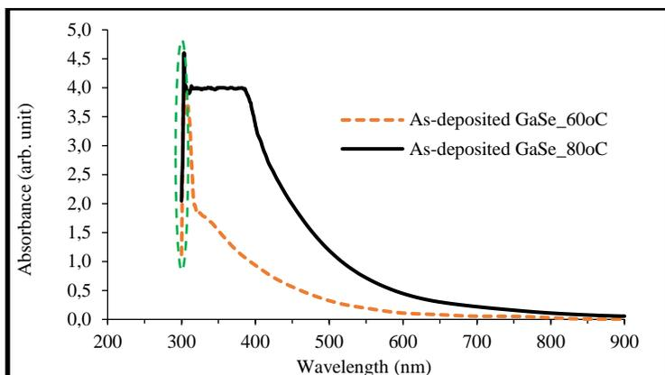
**Figure 1:** Optical absorbance graphs for as-deposited GaSe thin films. (Note that the dotted circled section represents the noise level at the ultraviolet region of the UV-visible spectrum)
