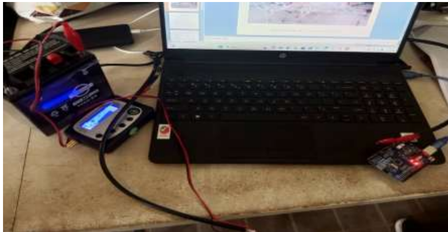
Fig 7 Indoor unit (Arduino board, Satellite Finder, 13V Battery and PC containing the necessary softwares- Arduino IDE and Stellarium)
